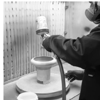
Spray painting room CMF library Coatings and textures Custom finishing for prototypes Sanding and engraving
