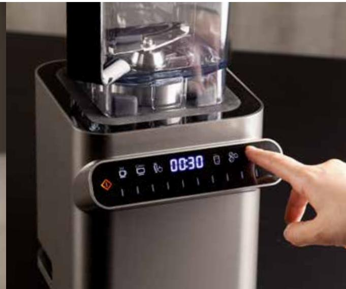
The interface required a specific study. It is a highly-evolved capacitive system that traces the finger movements without any perceived pressure. The innovation lies in the design of the command box that is mechanically distant from the jug that contains the blended food. This design prevents the liquids accidentally spilling onto the delicate electronic touch pad for the commands.
